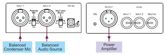
To connect up to two balanced audio sources to the 102xl 2 Channel Audio Mixer, do the following:
